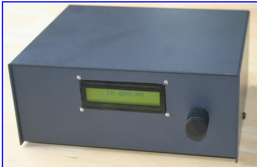
HC908 VFO mounted in optional Ten-Tec TPC-49 enclosure
