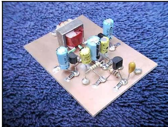
**Figure 12:** The completed homebrew Audio Amp assembly shows simple, effective use of SMT components used with conventional leaded components when constructed Manhattan-style.
