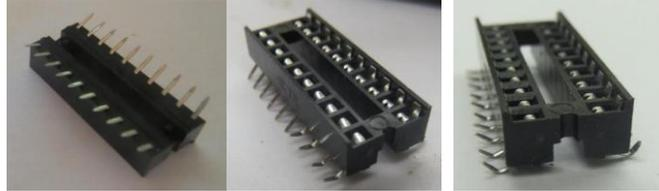
After the gull wing conversion, set the IC socket aside until all the small SMD parts have been soldered. The socket should not be installed now as it will be in the way of soldering the other parts and it may be damaged should you touch the plastic socket body with a hot soldering iron. Set it aside until all SMD parts have been soldered on.
