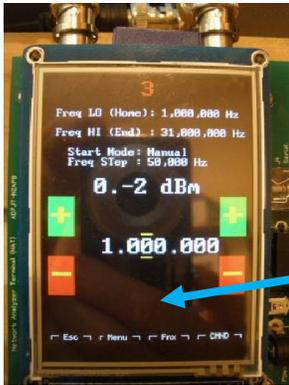
8. Tapping anywhere on the Freq Hi line will change the frequency to 31 MHz (note the change in signal amplitude).
