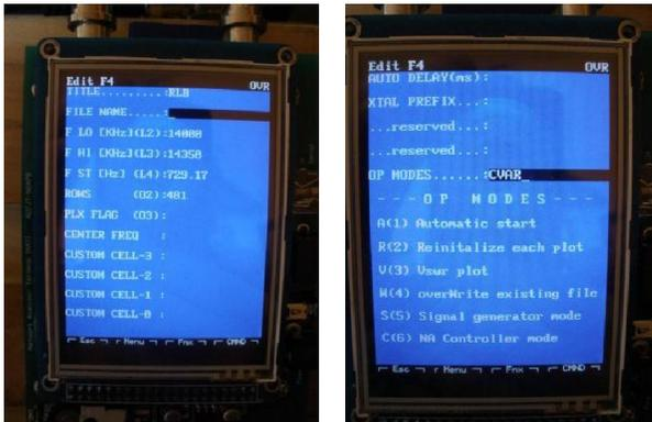
2. Press F4 to activate the PLX data sheet. The scan will start immediately and, after the initial scan, will repeat continuously. The time for each scan will depend on the number of frequency steps (FREQ ST) in the scan. In my case, with 481 frequency steps, each scan and plot takes about 0.8 seconds.
