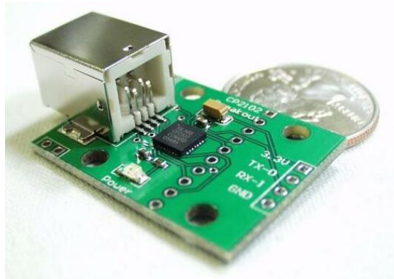
Photo 10: CP2102 USB-to-TTL interface from SparkFun
