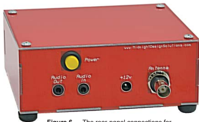
Figure 6 — The rear-panel connections for AUDIO IN/OUT, ANTENNA, and POWER.
