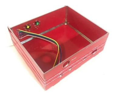
Solder both mating edges simultaneously using a blunt-tipped soldering iron while feeding generous amounts of solder to the joint. Low wattage is sufficient if you hold the soldering iron tip in place long enough.
