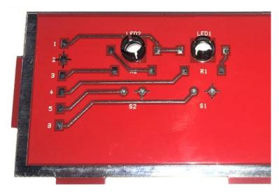
From the back of the Front Panel, push the two LEDs into the respective holder (green LED at the FT8 position, yellow LED at the ALT position). Using needle nose pliers or a flat blade screw driver, press the LEDs into the holder from the rear while holding the panel in your hand or against your leg. It will require strong effort, but the LED will eventually "pop" into the holder and protrude a little from it on the front side of the panel
